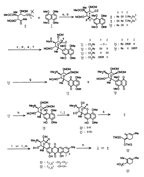
(a)  $\chi(1.4 \text{ eq})$ , n-BuLi(1.4 eq), THF, 0°C, 3 min, 57%(8), 4%(9), 22%(6) (b) Bu<sub>4</sub>NF, THF, r.t., 1 h, 98% (c) DMSO, (COC1)<sub>2</sub>, Et<sub>3</sub>N, CH<sub>2</sub>Cl<sub>2</sub>, -60-0°C, 95% (d) DIBAL, toluene, -78°C, 20 min, then K<sub>2</sub>CO<sub>3</sub>, MeOH, reflux, 30 min, 82% (e) MOMC1, (i-Pr)<sub>2</sub>NEt, THF, reflux, 3 h, 90% (f) LiAlH<sub>4</sub>,
